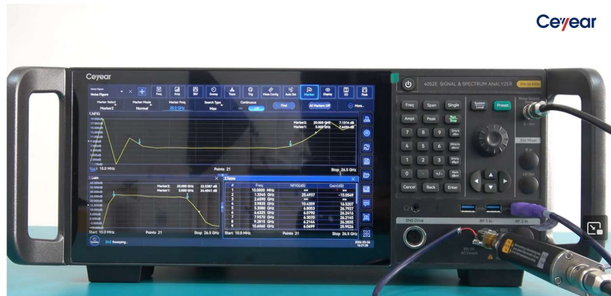
Figure 13. Viewing the Noise Figure measurement results with marker measurement capability.
