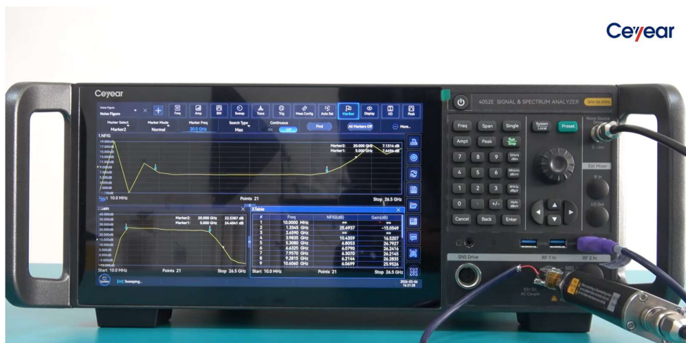
Figure 12. Noise Figure measurement in progress.
