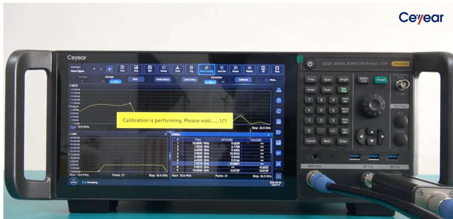
Figure 6. 6. System calibration in progress using the calibrated Noise Source.
