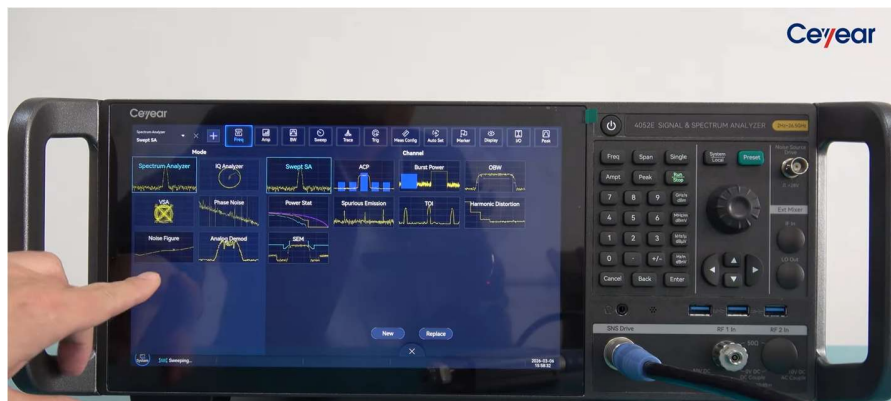
Figure 5. Ceyear 4052/4082 Signal & Spectrum Analyzer used for Noise Figure measurements.
