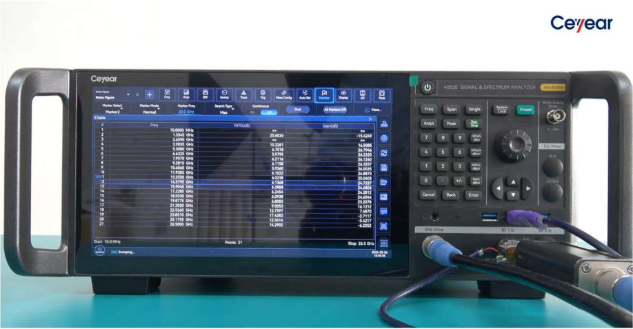
Figure 4. Automatic calculation of Noise Figure and Gain using the Y-Factor method.
